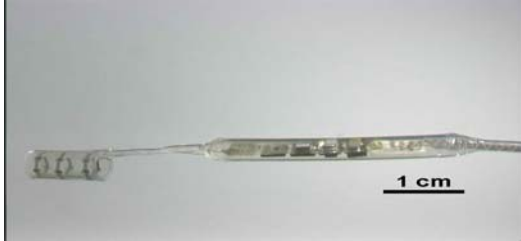
Figure 4: Modular assembly of a cuff electrode with multiplexer and Cooper cables.
